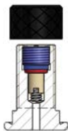
Model of valve stem integrated 7/8"14 UNF (C)
