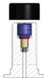
Model of valve stem integrated 5/8" 18 UNF (D)
