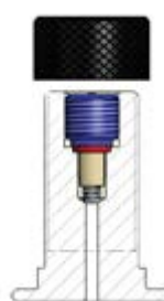
Model of valve stem integrated 5/8" 18 UNF (D)
